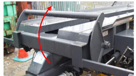
Make sure the container sub-frame contacts the trailer within the taper guides.
