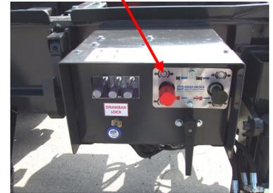
Correct engagement will allow the pin to drop into the locked position under pressure.
