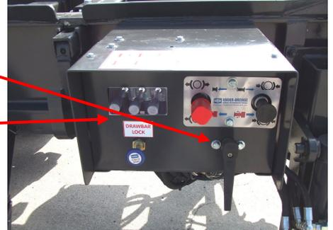
Level the trailer by operating the landing leg levers front & rear
