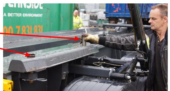
Replace the safety clips into the holding pins.
