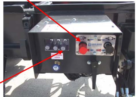
Using the lever, open the hydraulic container clamps on the trailer.
