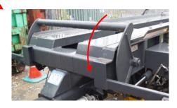
Engage the hooklift and pull the container onto the truck following the HOOKLIFT manufacturer's operating instructions.
